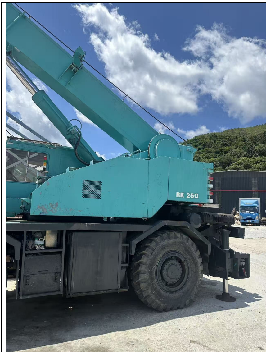
Figure 3: Side view of the KOBELCO RK250 crane and outriggers, demonstrating the need for a firm and level training surface.
